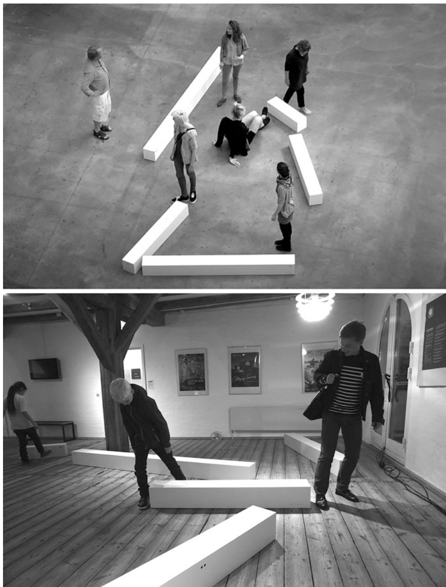
Fig. 10.1 © Cameline Bolbroe. Responsive prototypes in action in two different environments. These prototypes respond to motion in their vicinity via ultrasound sensors. When participants trigger the sensors, the beams move around via embedded motors. The beams have varying motion patterns so that three of them move around a pivot point at one end, whereas the other two move transitionally
