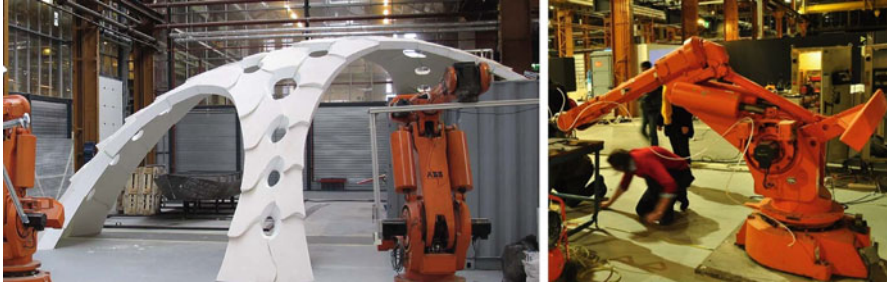
Fig. 12.6 Prototype built by means of robotic wire cutting in a wire cutting in a Hyperbody off-campus lab (2012)
