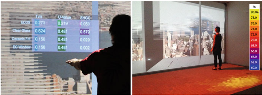
Fig. 11.4 A pop-up data panel displays real-time performance values for the adaptive facade system ( left ). The large-screen simulation environment displays a full-scale analysis map on the floor in colors representing daylighting or heat gain ( right )
