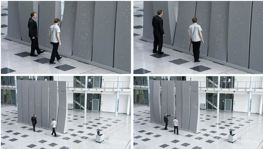
Fig. 12.2 Interactive Wall developed by Hyperbody in collaboration with Festo responds to people's movement (2009)
