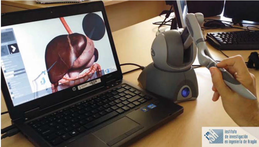
Fig. 3.8 A virtual surgery simulator based on the same algorithm explained in this chapter
