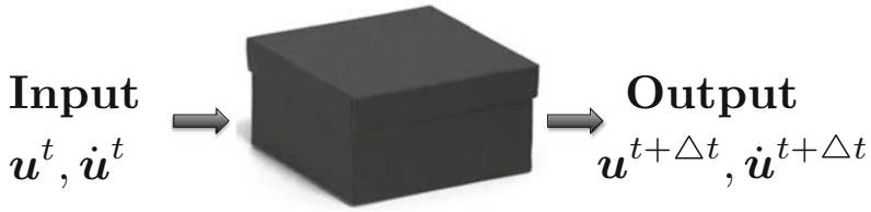
Fig. 5.1 Sketch of the proposed method for the integration of solid dynamics in the PGD framework. Converged displacement and velocity fields at time step t are taken as parameters, so as to provide, without the need of any matrix inversion, the displacement and velocity fields at time step t + \Delta t
