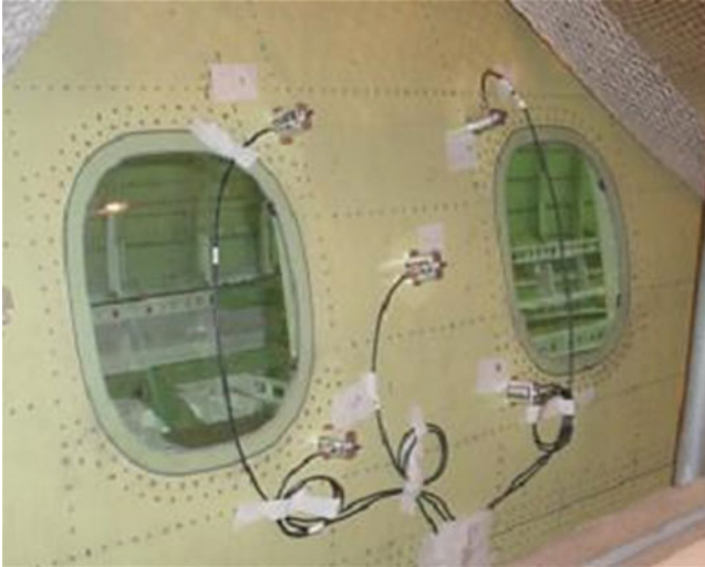
Fig. 10 Fuselage panel in the E-Jets FSFT monitored by acoustic emission
