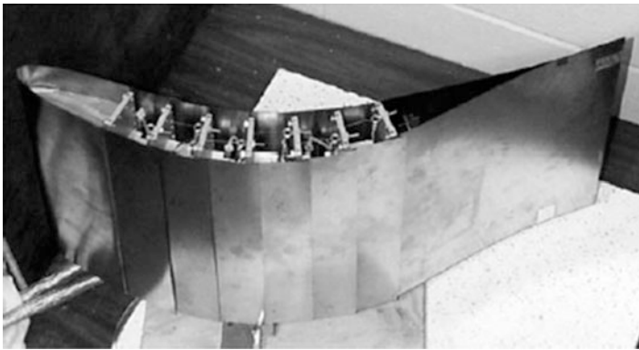
Fig. 5 SMA multi-actuated hydrofoil prototype (Rediniotis et al. 2002)
