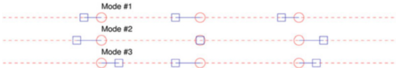
Fig. 26 Schematic representation of the vibration modes of the 3-dof spring–mass system
