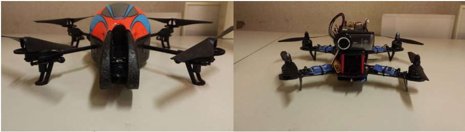
Fig. 11. Left: AR Drone with forward looking camera. Right: XBird with webcam attached on the frame.
