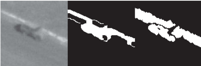
Fig. 4. From left to right: Original image, Canny edge detection results, MSER detection results. Figure illustrates an important advantage of MSER detection over Canny edge detection that is its ability to separate regions by their intensity difference.
