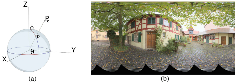
Fig. 1. (a) Spherical coordinates and illustration of the spherical projection. (b) Pixel-map of a spherical image.
