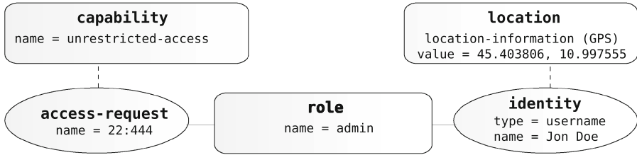
Fig. 1. Example MAP graph: ellipses represent identifiers, rectangles represent metadata, both of which are modeled as different types of nodes. Edges represent relations between identifiers and metadata. In this representation, links are implicitly shown via their attributed metadata connecting two identifier nodes, such as role .
