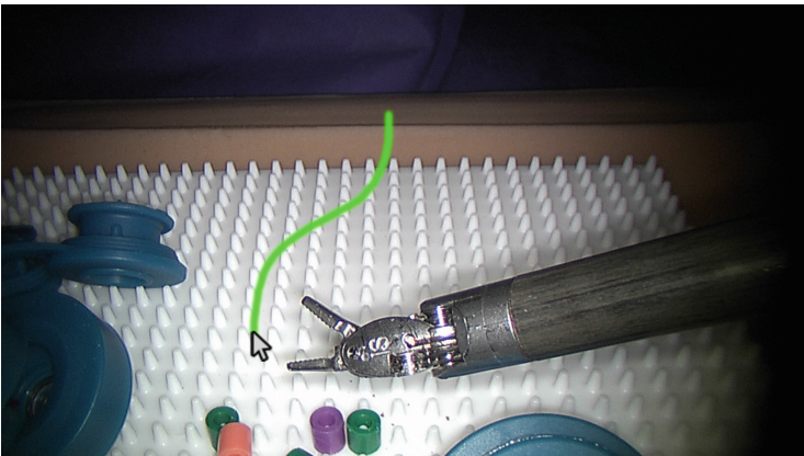
Fig. 2. The cursor and a line drawing overlaid on one of the video channels of the da Vinci S HD system. Note that a monoscopic image cannot convey the appearance of a one-eyed cursor.
