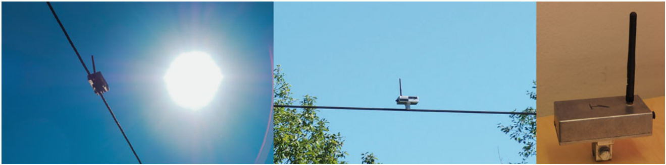
Fig. 15.3 The catenary sensor consists of up to ten motion-processing units (MPU) as shown
