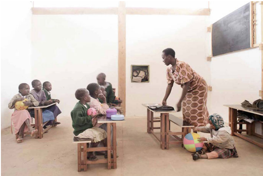
Fig. 8.4 Classroom with the self-produced furniture. The high windows combined with white plaster allow good natural lighting without glare (Source: Image by Live in Slums NGO)
