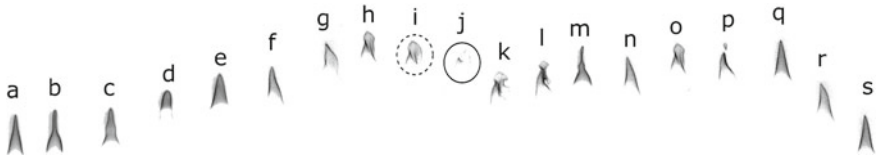
Fig. 17.8 Flame dynamics during intermittent oscillations are shown through instantaneous images. Images are arranged in the order of their occurrence ( left to right ). Circles on the instantaneous images highlight the characteristic stretching, folding ( i ), and local extinction ( j ) in the flame
