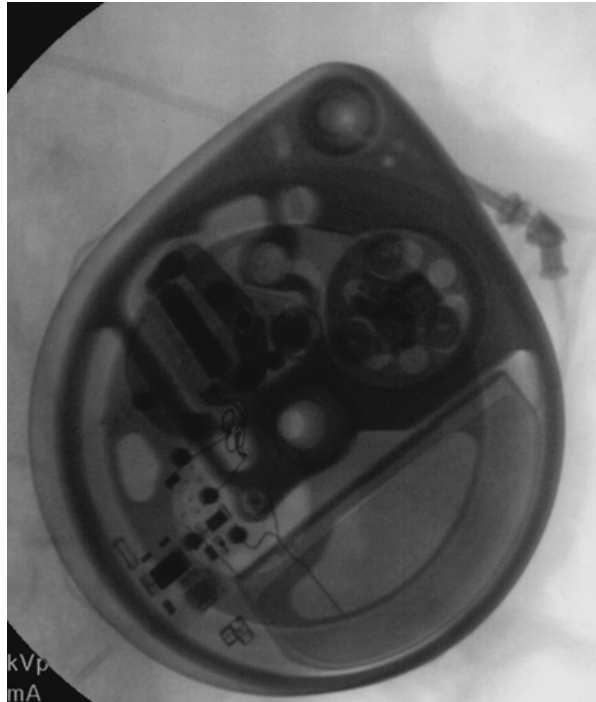
Fig. 7.11 Image of a surgically implanted intrathecal pump (Courtesy of Andrew Engel, M.D.)
