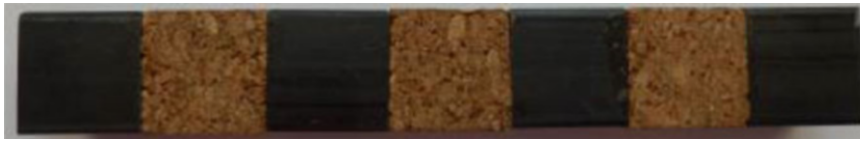
Fig. 14.1 Two-material PIVI device for longitudinal vibration attenuation
