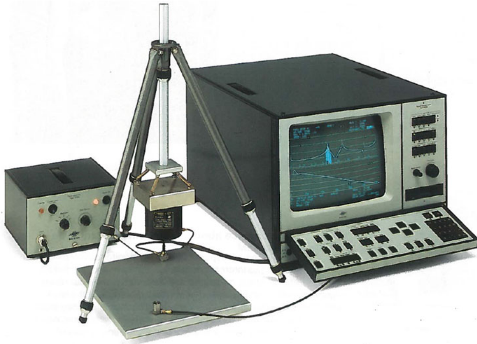
Fig. 4.1 Multichannel Analysis System Type 3550 with a typical dual channel mobility shaker setup
