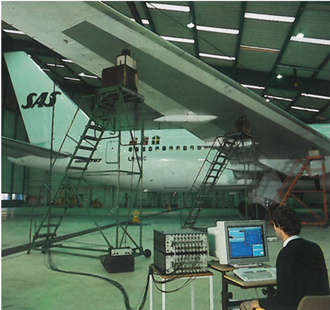
Fig. 4.2 MIMO based on a 16 channel Type 3550/3551 system
