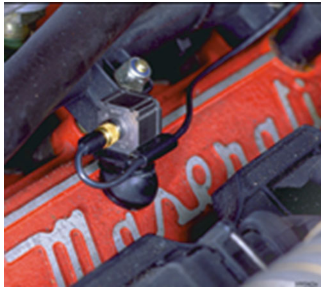
Fig. 4.6 Tri-axial accelerometer Type 4506 mounted on a swivel base
