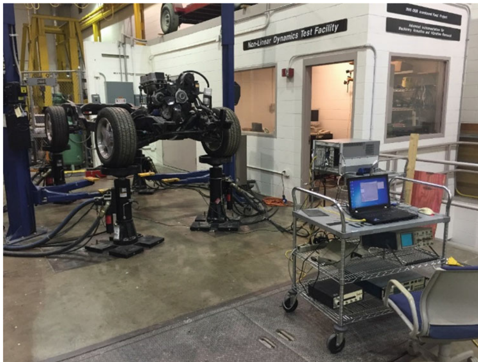
Fig. 6.11 Experimental test setup using pick-up truck frame
