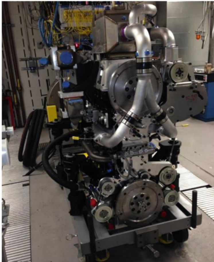
Fig. 3.1 Achates Power A48-3 opposed piston two-stroke engine
