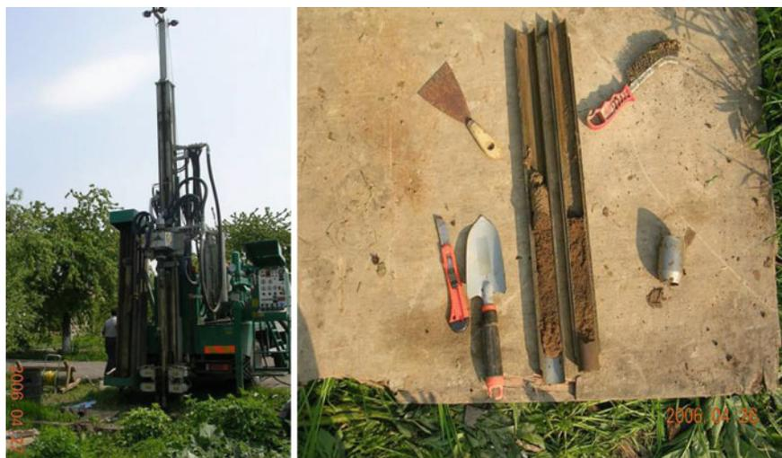
**Fig. 5** Standard penetration technique (equipment and sampling)
