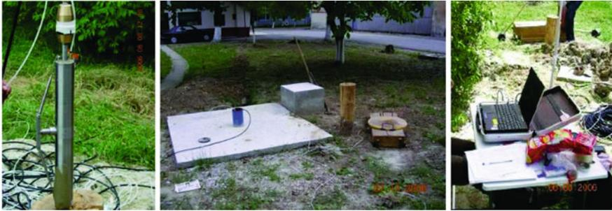
**Fig. 2** PS Suspension logging system (down-hole technique)
