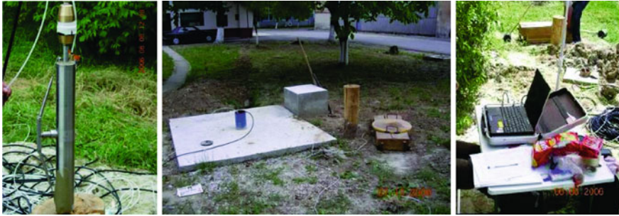
Fig. 2 PS Suspension logging system (down-hole technique)
