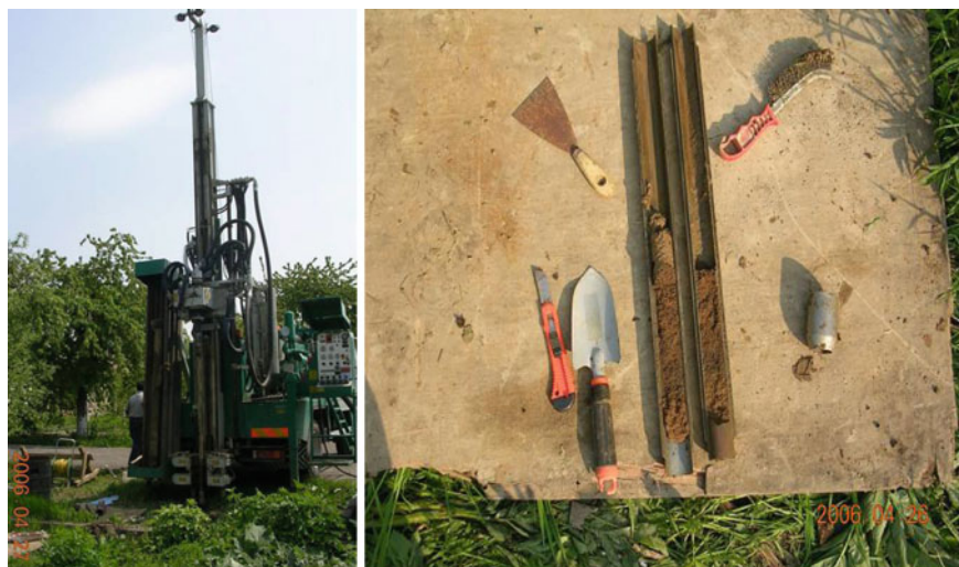
Fig. 5 Standard penetration technique (equipment and sampling)
