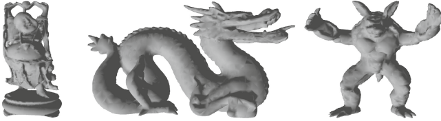
Fig. 4. Simplifications of the model Armadillo, Dragon and Happy Buddha (93%–95% of triangles removed) from the Stanford 3-d scanning repository
