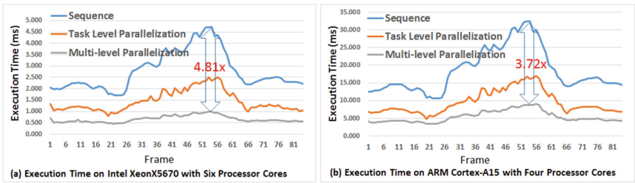
Fig. 7. Execution time per a frame for the road tracking application on Intel and ARM multi-cores
