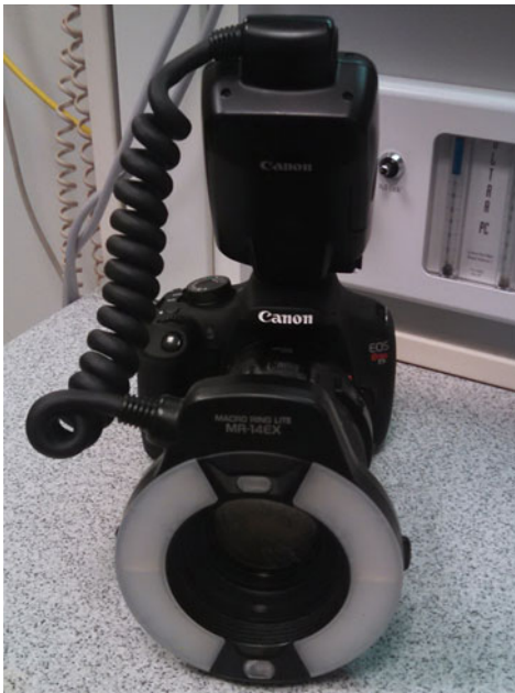
Fig. 3.12 Digital SLR camera equipped for intraoral photography with macro lens and ring flash
