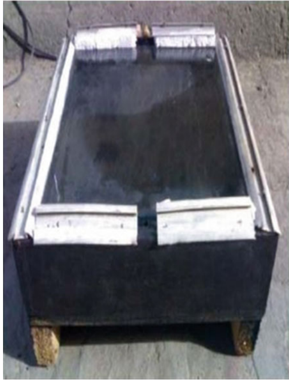
Fig. 5 Direct absorption solar collector (Verma and Kundan (2013))
