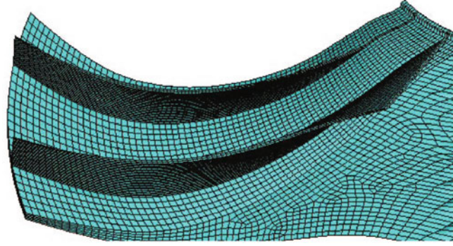
Fig. 8.1 Part of the finite element mesh of the bladed disk
