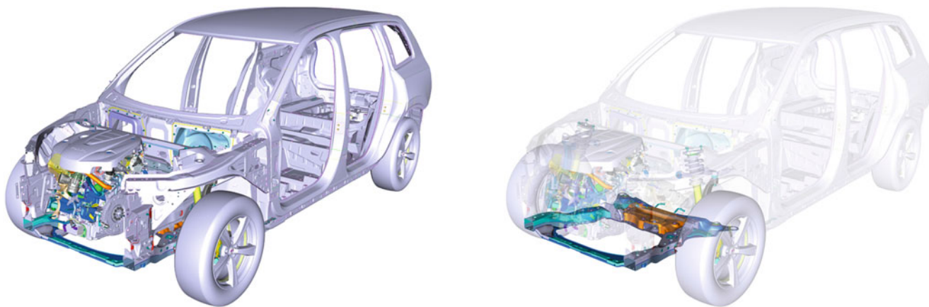
Fig. 31.1 The front subframe is an important part from a vibration perspective as it connects the suspension link arms and engine to the car body. (a) Parts of an XC90; (b) Front subframe location in the car
