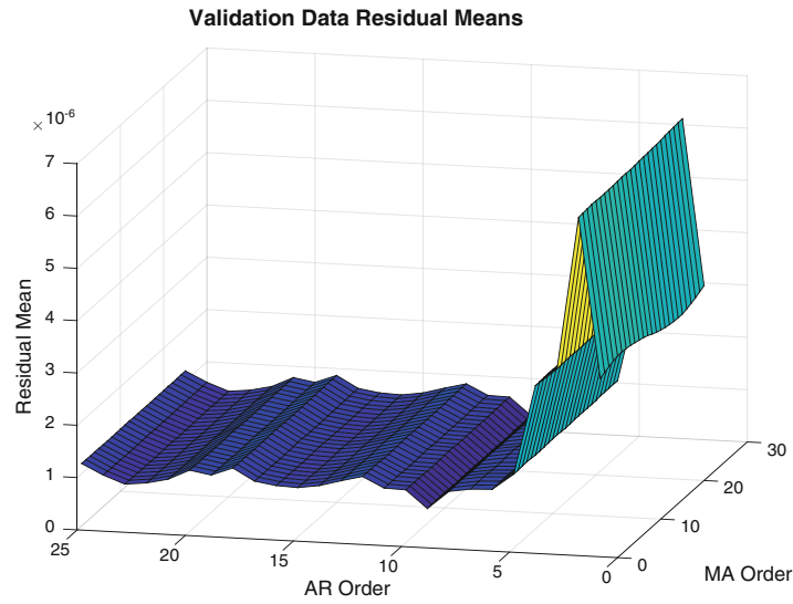
Fig. 13.2 Mean values of ARMA residual errors for varying model orders (N; M)
