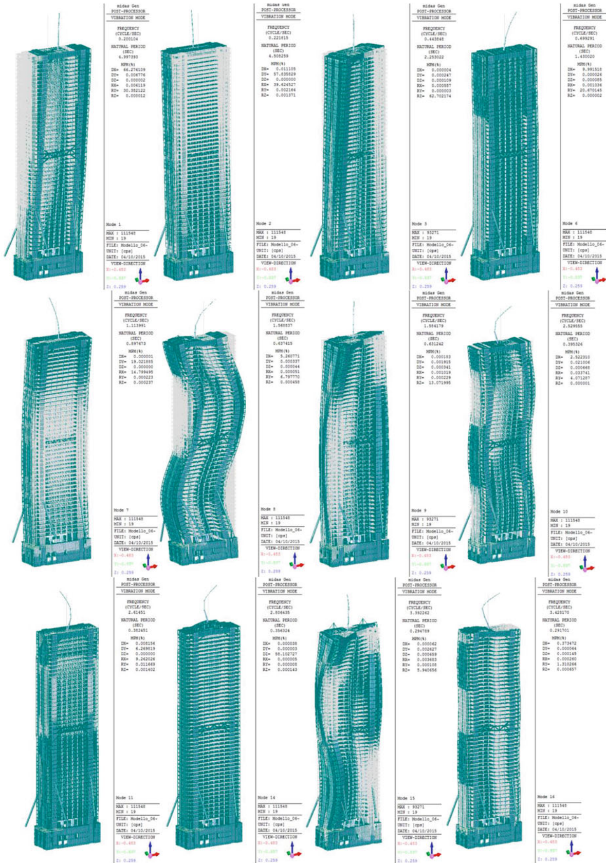
Fig. 32.3 Mode shapes of the first 12 vibration modes of the Allianz Tower, as derived by eigenvalue analysis
