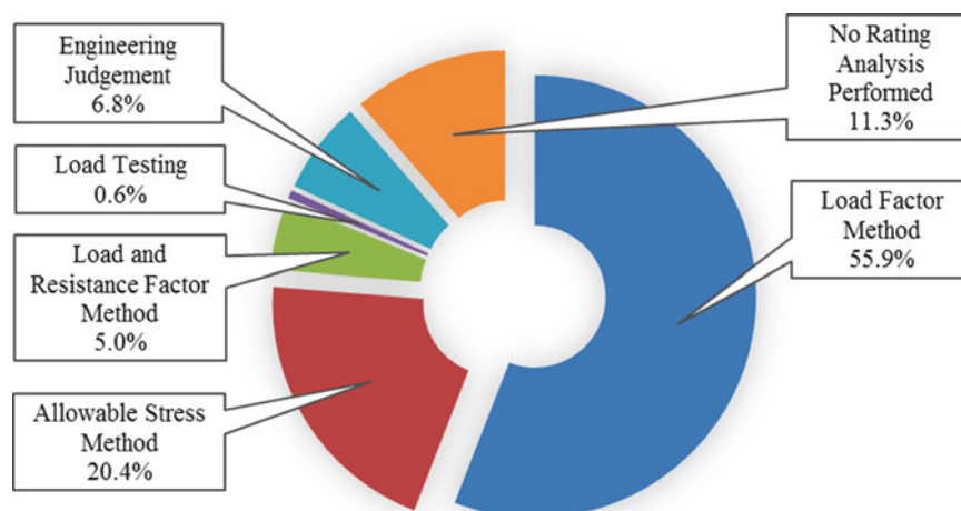
Fig. 18.1 Load ratings methods used for US bridges
