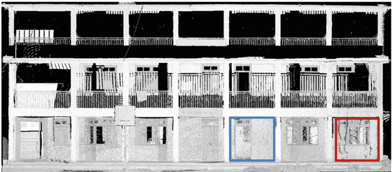
Fig. 5.6 Front view of the point cloud (the two -red and blue- rectangles indicate location of the exterior and interior walls, respectively)
