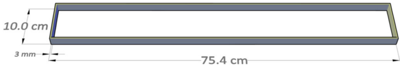
Fig. 29.6 Dimensions of the flexible frame
