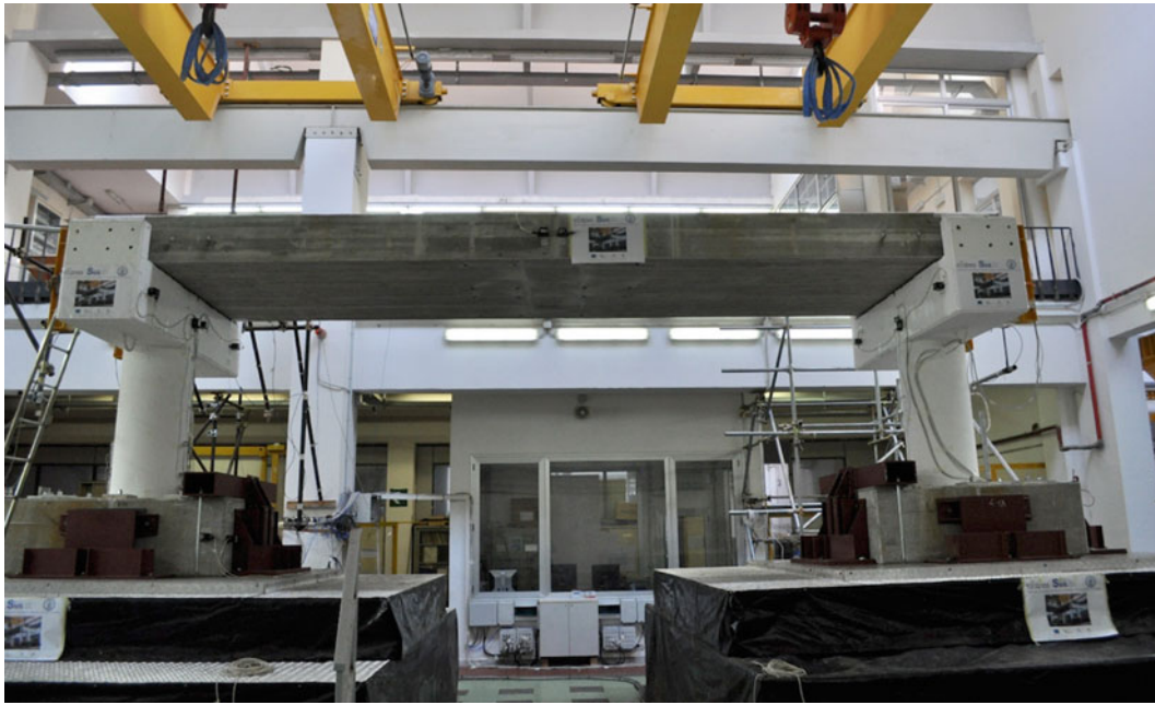
Fig. 20.1 The testing configuration of the bridge model
