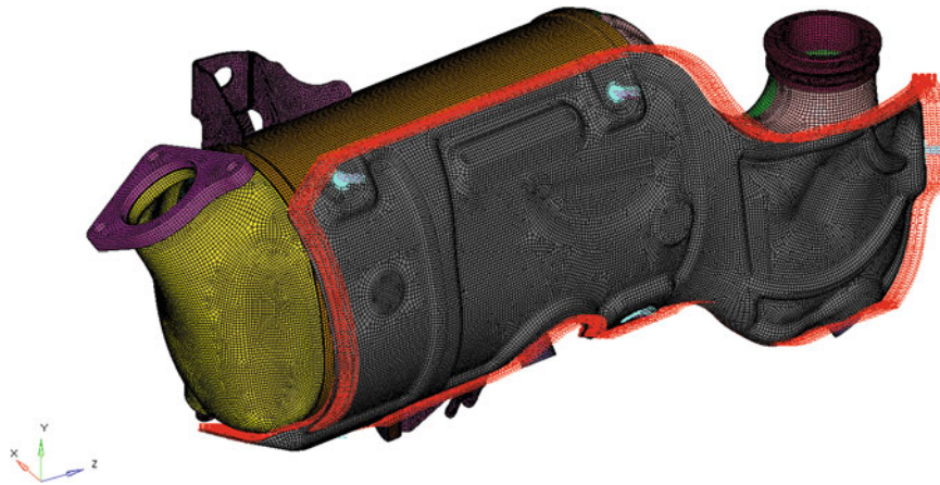
Fig. 16.8 Full FEM model of the constrained heat-shield
