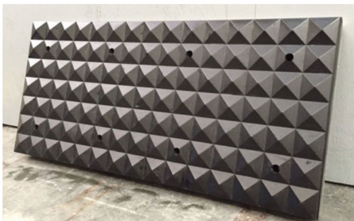
Fig. 13.4 Urethane programmer used as a loading medium to transfer and tailor the shock pulse applied on the specimen. The front face has a pyramidal geometry which was specifically designed to achieve a shock pulse similar to that of a blast load
