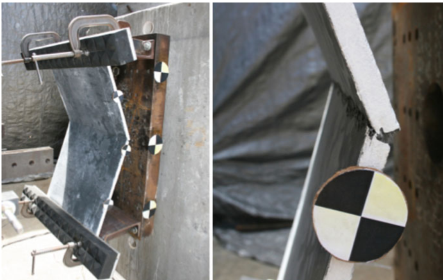
Fig. 13.7 Behavior of sheathing including midspan hinge development when subjected to increasing levels of simulated blast loads using hydraulic blast generator
