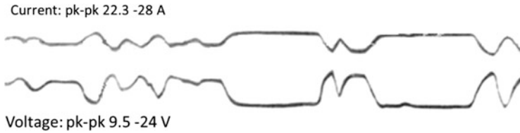
Fig. 9.9 Current and voltage waveforms for short air gap hissing mode. The voltage peak-to-peak varies between 9.5 and 24 V and the current peak-to-peak varies between 22.3 and 28 A
