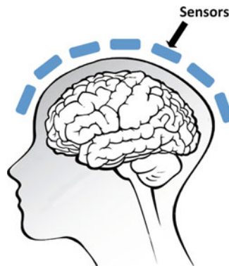
Fig. 25.3 fMRI and MEG recordings. In these recording techniques, electrodes are located at a distance from the head. In addition to its high spatial resolution, fMRI makes it possible to acquire signals from subcortical regions. Conventional fMRI machines suffer from very poor temporal resolution, a property which makes this method less suitable for real-time experiments. MEG, on the other hand, is a sophisticated device that obtains relatively high spatial and temporal resolutions. Major drawbacks of fMRI and MEG as components of NF system are lack of portability, high price of facilities and restrictions imposed on the subjects while recording (Figure adopted from http://image.shutterstock.com/z/stock-vector-human-brain-medical-schematic-simplified-illustration-on-white-74522395.jpg )
