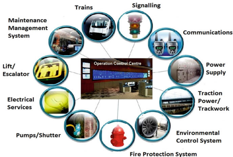
Fig. 1 The composition of a modern MRT
