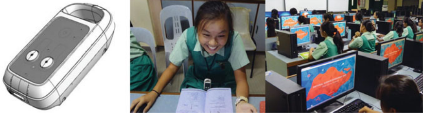
Fig. 1 The third generation SENSg device ( left ) which is worn by students on a lanyard ( center ) which allows them to explore their personal travel and environmental data ( right )
