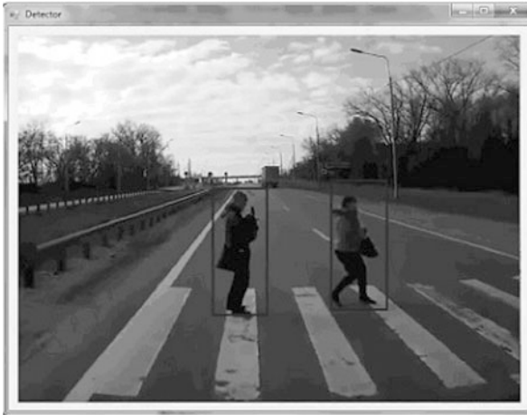
Fig. 3 Demonstration of the Haar features-based pedestrian detection
