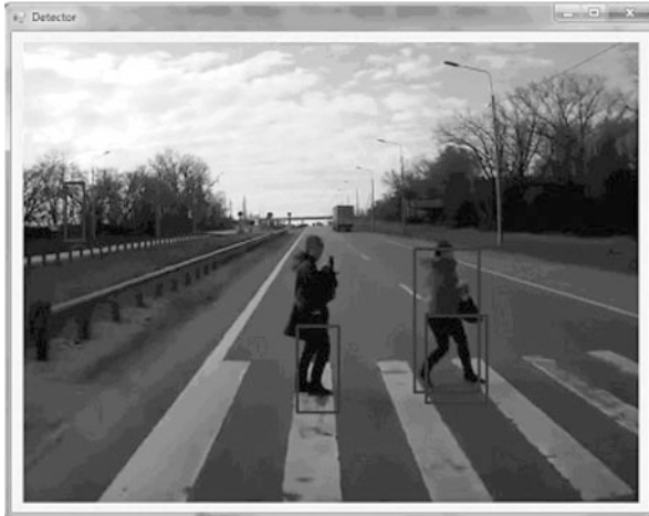
Fig. 1 Demonstration of the HOG-based pedestrian detection
