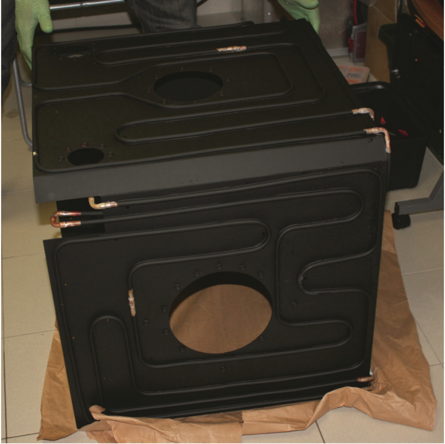
Fig. 2. The liquid nitrogen cooled shroud removed from the chamber, with the brazed copper coil visible.
