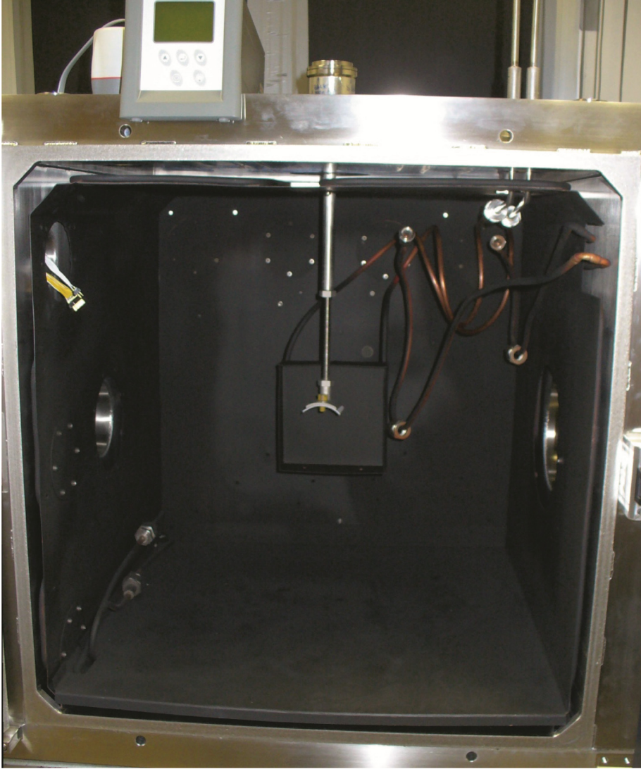
Fig. 1. Internal test volume of the vacuum chamber. The five walls visible in black are painted with Aeroglaze Z306. A smaller nitrogen cooled shroud, used for some tests, is visible just behind the small shaft that is attached to the rotational manipulator at the top of figure.
