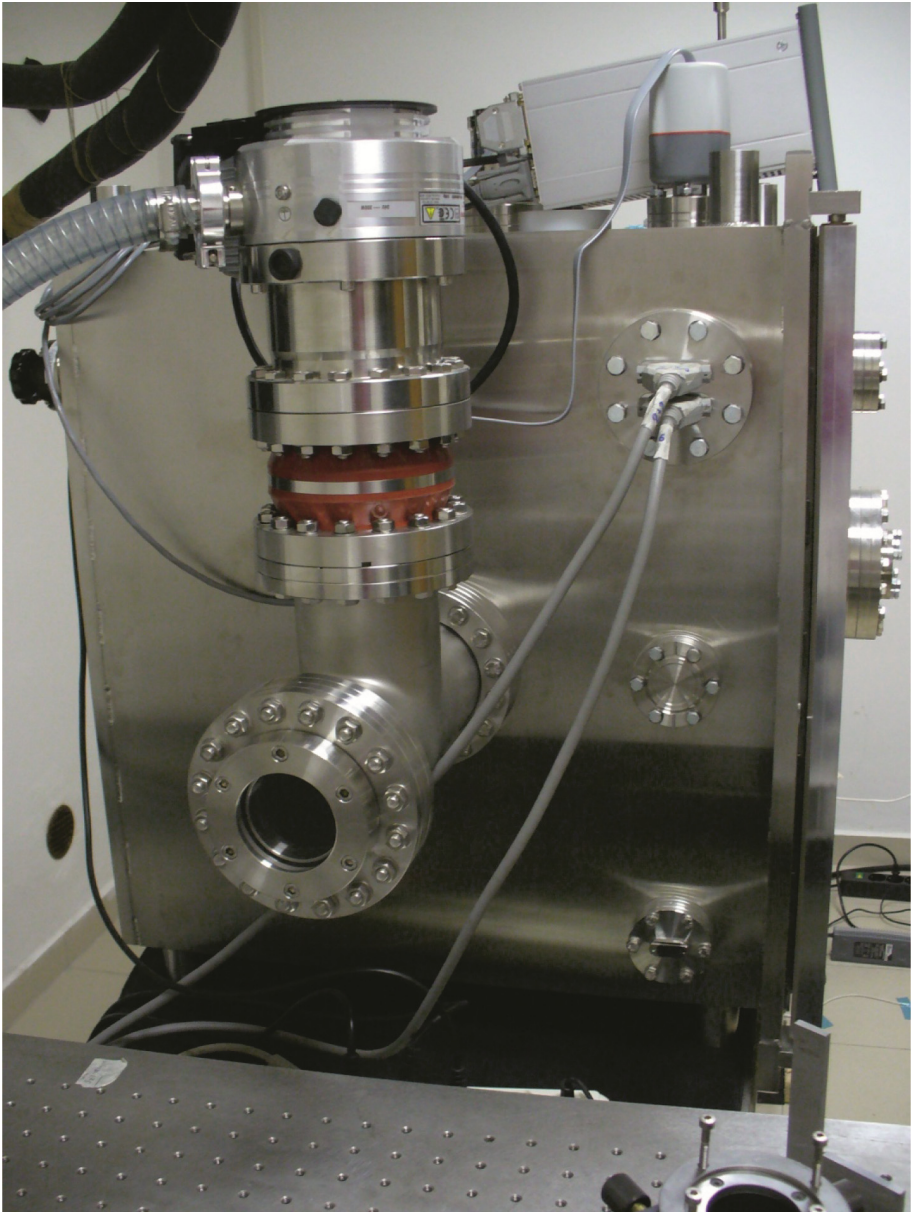
Fig. 6. The high precision optical window for optical testing. Above the window is mounted the turbo molecular pump over a vibration damper (in red). The same side of the chamber hosts the electrical feedthroughs (top and bottom right) (Color figure online).
