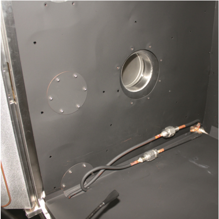
Fig. 4. The Swagelok fittings can be used to remove the cooled floor of the shroud if needed, to test heavy specimens.
