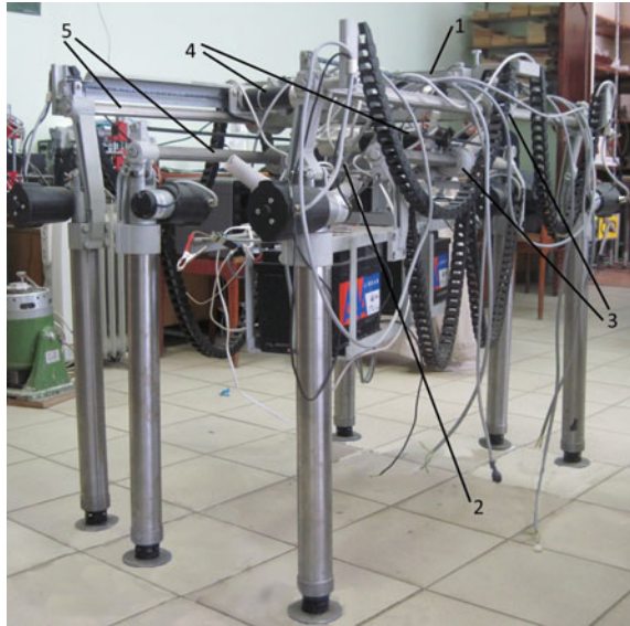
Fig. 1 Robot movements with orthogonal drivers: 1 upper body, 2 lower body, 3 guide sleeves, 4 driver of the horizontal movement, 5 robot frames with support columns
