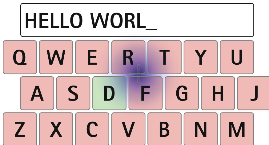
Fig. 6.6 In a touch screen keyboard, a language model provides a probability for the next letter (shown here as key color) and a touch model gives a measure of certainty for a user’s touch (here shown as a gradient around the touch position indicated by a cross). The combination of both models determines the most likely next letter. We vary how much influence the language model has by changing the size of the touch area. When users press harder, it shrinks and keys closer to the touch are much more likely to be chosen. As users relax and only press lightly, the area increases and many more keys are potentially chosen—increasing the influence of the language model
