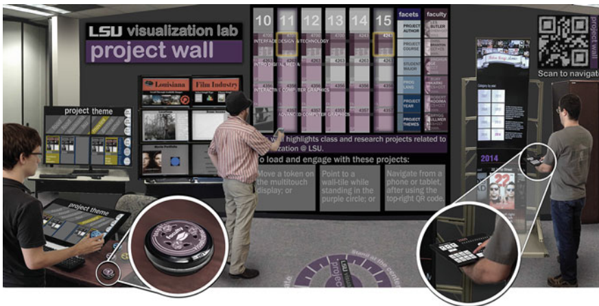
Fig. 12.6 Frey visualization laboratory wall envisionment: Three tiled displays (in 2 \times 2 , 3 \times 2 , and 1 \times 2 configurations) have long been installed for researcher and classroom use. Building on responses to the Coates hall envisionment, some aspects are envisioned as retained. The 3 \times 2 and 1 \times 2 tiled displays present student projects. These are illustrated as selected via tangible interaction with a 27" multitouch monitor on the bottom left , the contents of which are mirrored on the 2 \times 2 tiled display
