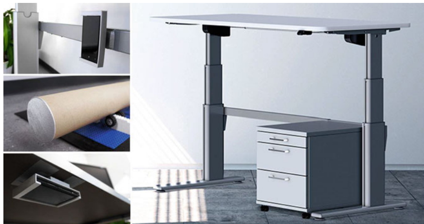
Fig. 9.8 Prototypes for peripheral interaction through smart furniture: smart furniture modules for under-the-desk kicking, rolling, and touching
