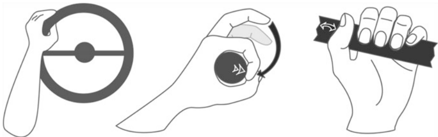
Fig. 5.10 The steering wheel setup ( left ) allows for easily perform microgestures ( center, right ), which could turn any automotive, mobile device, or wearable device control into a microinteraction that is done as secondary or peripheral task during driving
