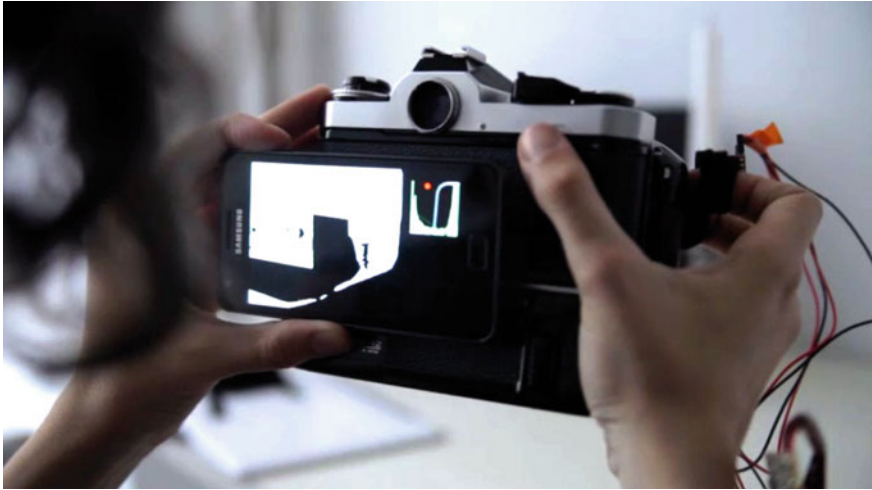
Fig. 5.12 An Android-running camera application is controlled through microgestures that are performed wherever the fingers are best placed to hold the device, without any restriction of the position of physical or digital buttons
