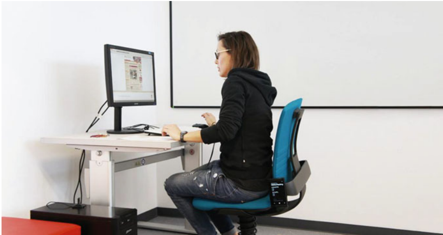
Fig. 9.7 Prototype for peripheral interaction through smart furniture: interactive office chair
