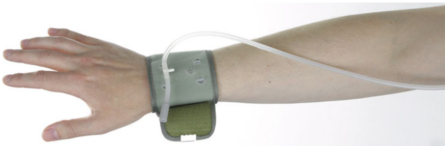
Fig. 6.7 We are experimenting with pneumatics in cuffs around the wrist to apply compression feedback as a modality for low-disruption background notifications
