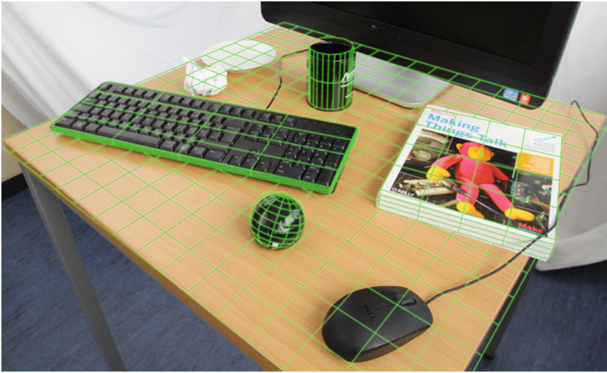
Fig. 6.4 Instead of embedding input capabilities into objects around us, we can leave them as is and track them externally. Manipulations of such objects or touches on them can then be used as a means of input. We can, for example, temporarily make a nearby coffee mug a volume slider or press down on a hacky sack to use it as a transient button. Such appropriation of objects can be limited to a given interaction window (e.g., the hacky sack is only a button when a call is coming in), or persist over longer durations (when objects are explicitly set aside for specific interactions)
