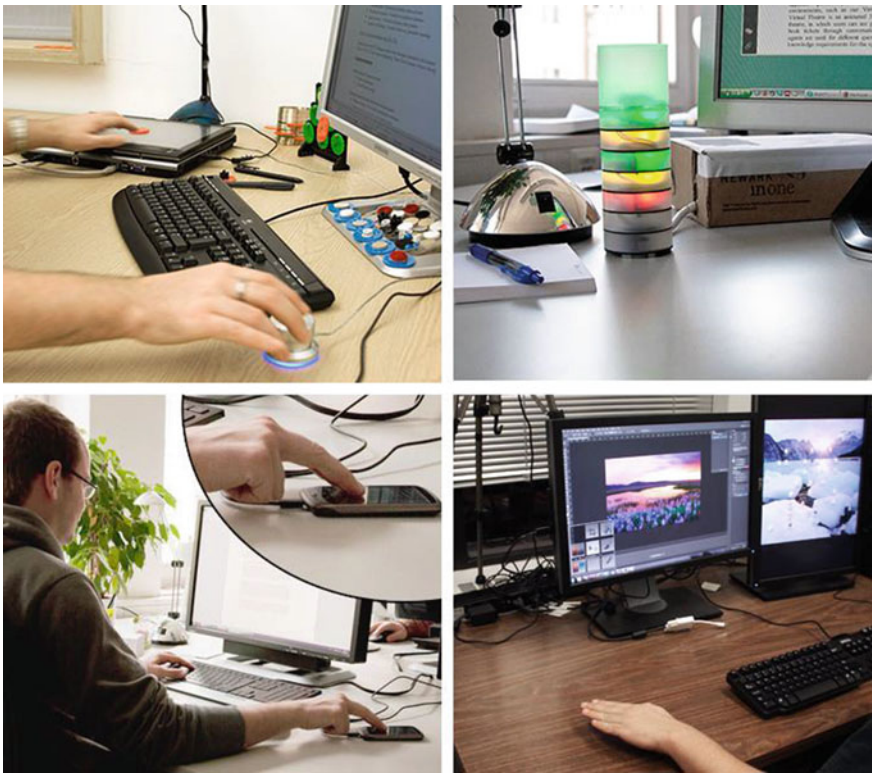
Fig. 9.5 Examples of peripheral interaction in desktop scenarios: office-based peripheral TUI (Edge 2008), StaTube tangible presence indicator (Hausen et al. 2012), peripheral music controller (Hausen et al. 2013b), and Unadorned Desk extended input canvas on a physical desk (Hausen et al. 2013a)
