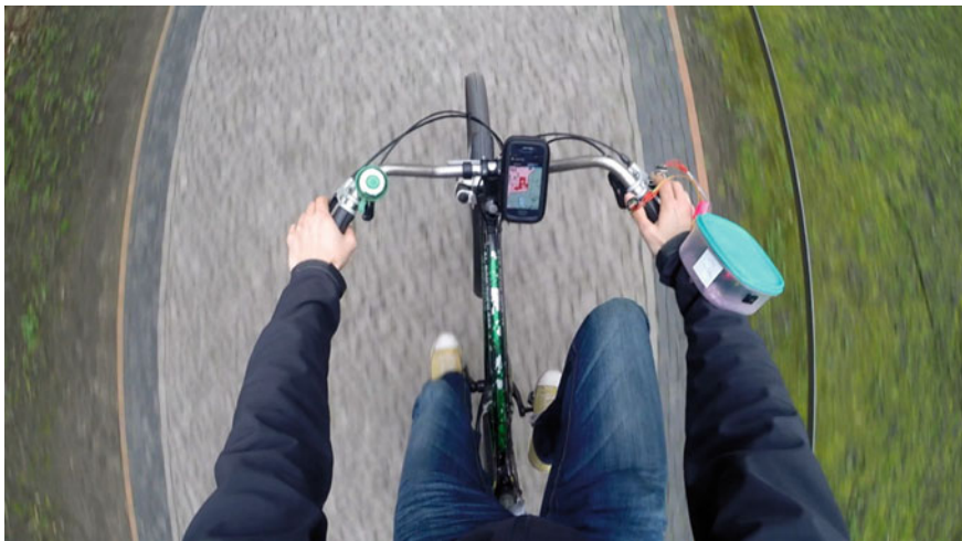
Fig. 5.1 Smart cycling through wearable sensors that detect microgestures allows for navigating through a map without releasing the handle bars
