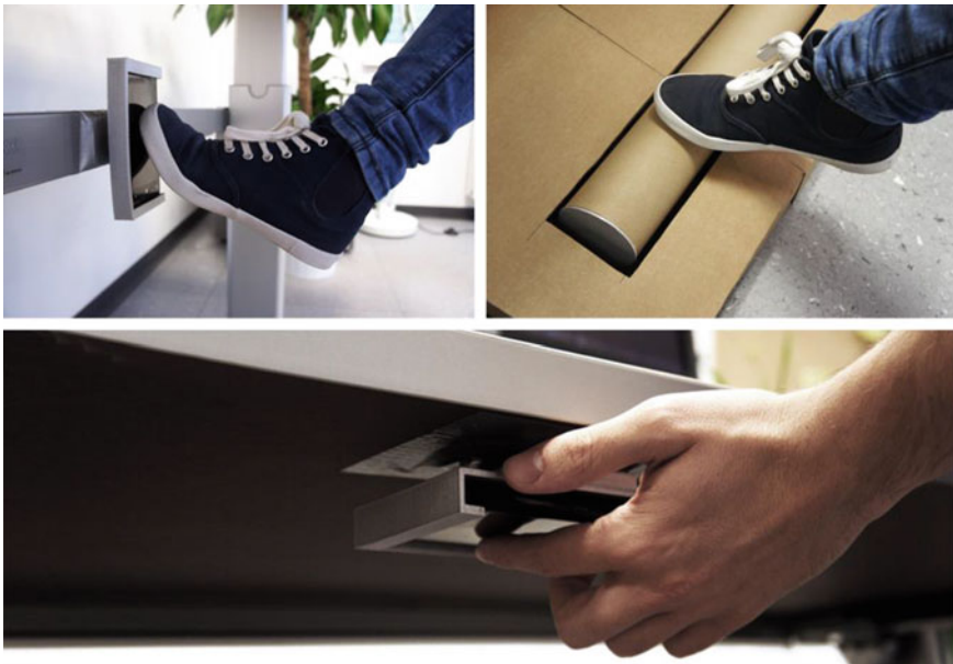
Fig. 9.11 Peripheral interaction through smart furniture, under-the-desk foot, and hand gestures
