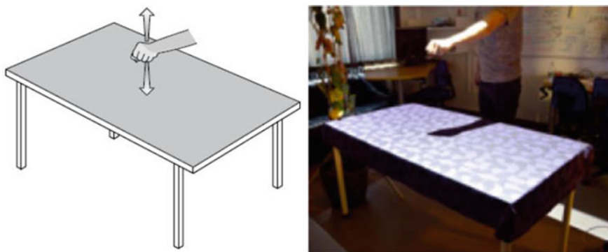
Fig. 10.12 Controlling brightness by moving hand up or down (Andersen and Sørensen 2014)
