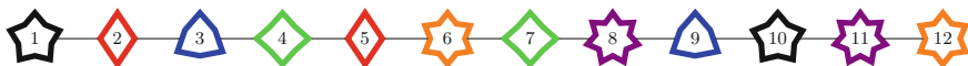
Fig. 4. The greedy algorithm might choose to color the path (2, 3, 4, 5), then it must recolor one of the vertices {1, 10}, one of {6, 12}, and one of {8, 11}, a total of five recolored vertices, while an optimal recoloring can recolor the paths (4, 5, 6, 7) and (8, 9, 10, 11), a total of four recolored vertices (Color figure online).
