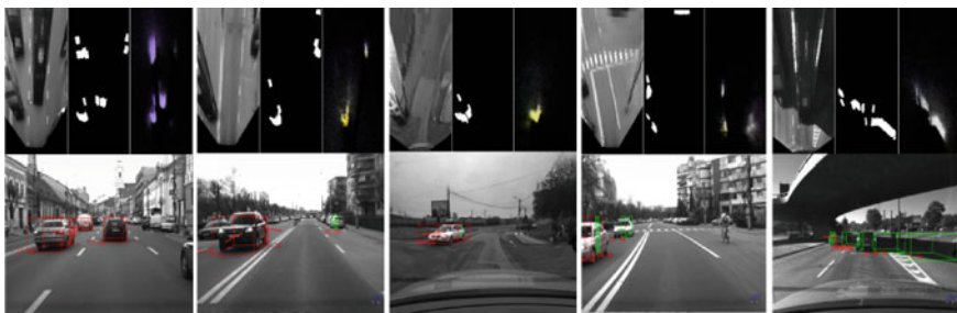
Fig. 6 Successful detection for cars of multiple orientations, and pedestrians ( panels 1, 2 and 3 ); a detection failure ( panel 4 ), and false positives ( panel 5 )
