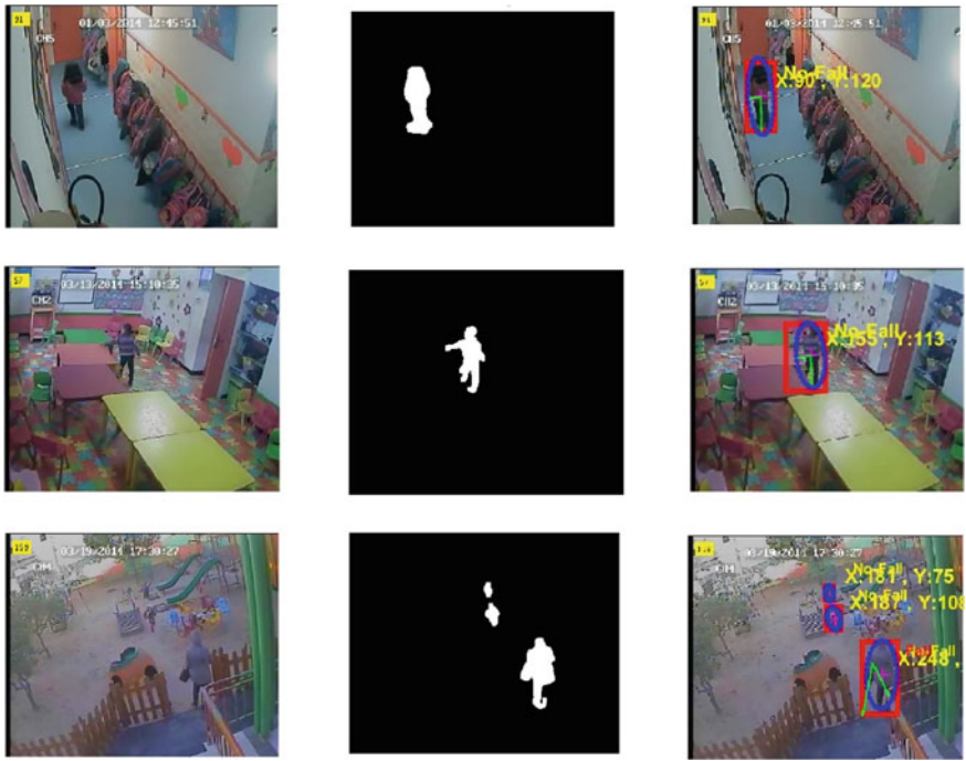
Fig. 6 First column Video frame. Second column Human silhouette. Third column Experiment results of fall detection
