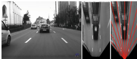
Fig. 2 Removal of the perspective effect. The obstacle areas will expand radially from the camera position point
