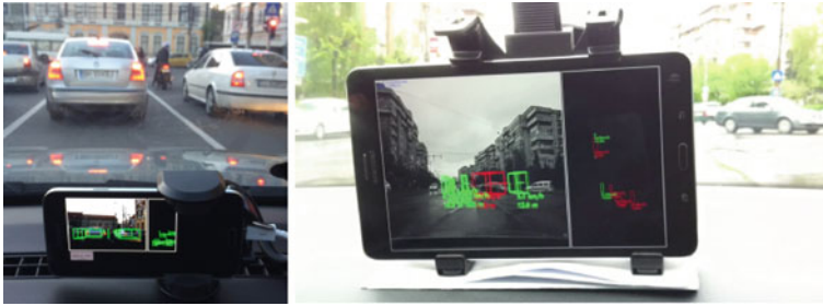
Fig. 7 Obstacle detection using a smartphone ( left ) and a tablet ( right ), mounted inside the vehicle
