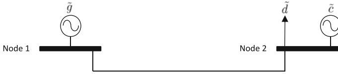
Fig. 3.3 Illustrative Example 3.7: two-node electric energy system
