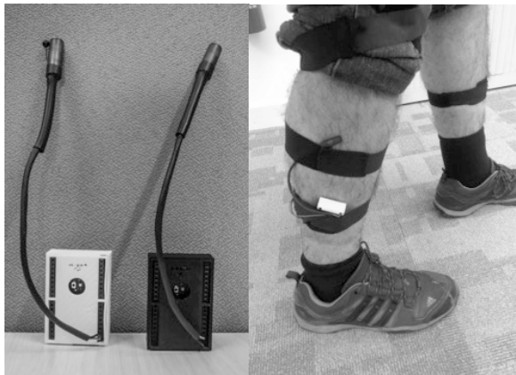
Fig. 2 Last user-tested version of the Haptic Bracelets (left). A Haptic Bracelet device strapped on a user's leg (right).
