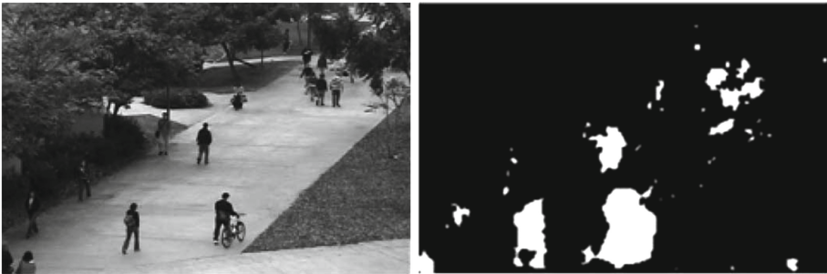
Fig. 4. Foreground segmentation using optical flow. Left: Input sample from the PEDS dataset. Right: Segmented foreground
