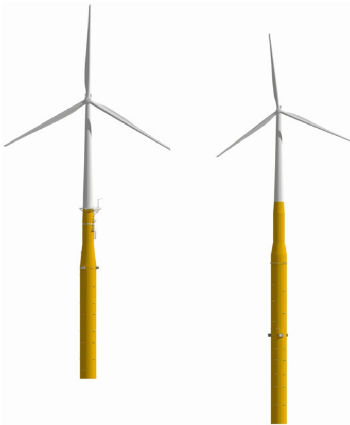
Fig. 14 Hywind 6 MW design ( left ) and Hywind Demo ( right ) (courtesy of Statoil)
