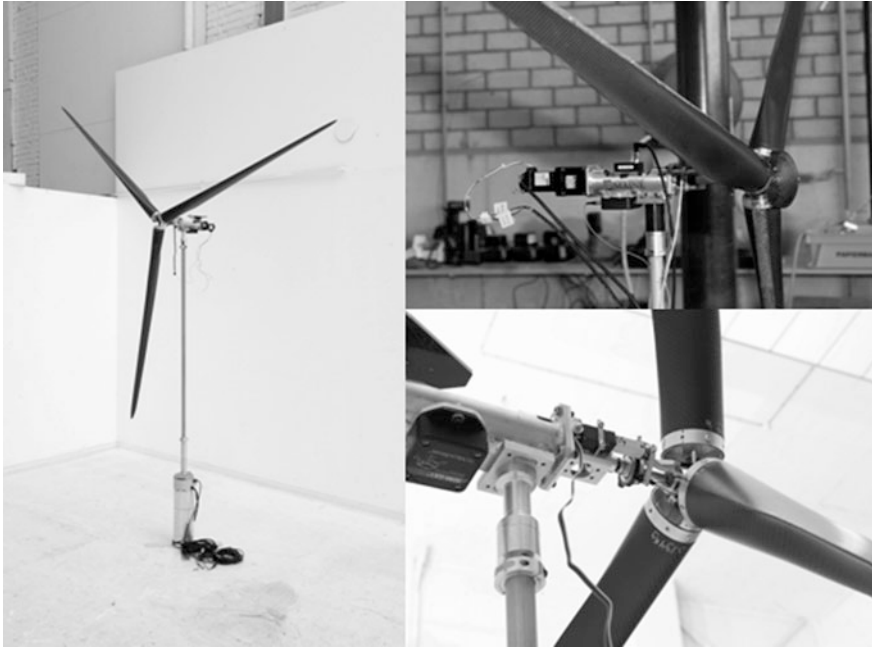
Fig. 43 Image of 1:50-scale model wind turbine used in DeepCwind model test campaign
