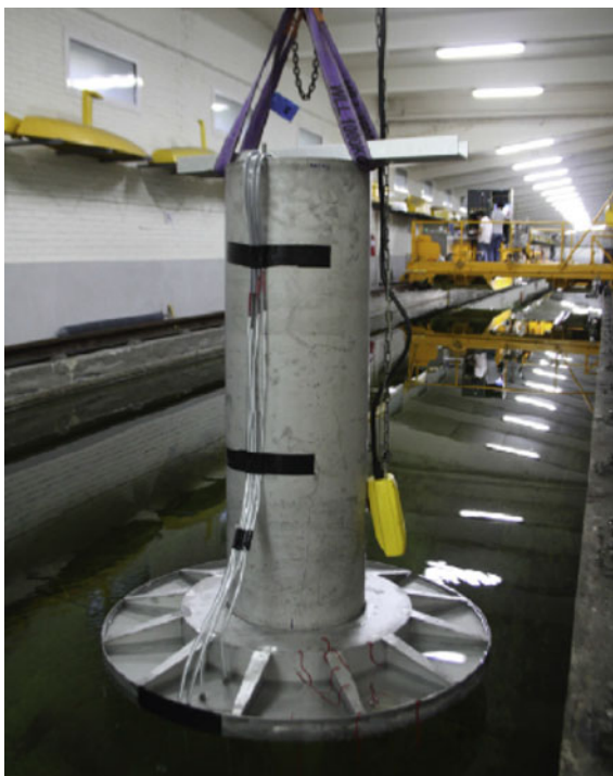
Fig. 14 Photograph of the experimental model used in Lopez-Pavon and Souto-Iglesias (2015)
