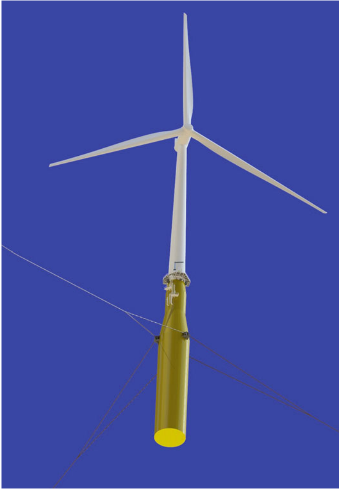
Fig. 12 Hywind deep spar concept (courtesy of Statoil)
