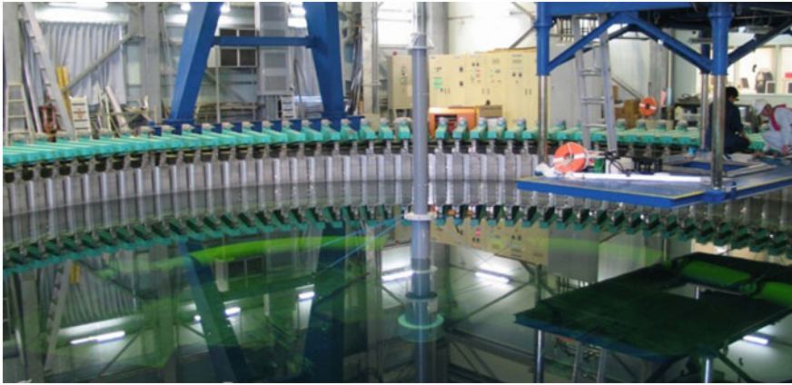
Fig. 31 1:22.5 scale model of the 2 MW prototype model in the deep sea wave basin at National Maritime Research Institute (Japan)
