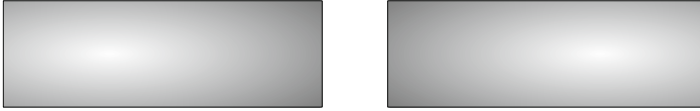
Fig. 2.9 Proximity effect in two closely spaced lines. Current density distribution in the cross section of two closely spaced lines at high frequencies is shown in shades of gray . Darker shades of gray indicate higher current densities. In lines carrying current in the same direction (parallel currents), the current concentration is shifted away from the parallel current. In lines carrying current in opposite directions (antiparallel currents), the current concentrates toward the antiparallel current, minimizing the circuit inductance
