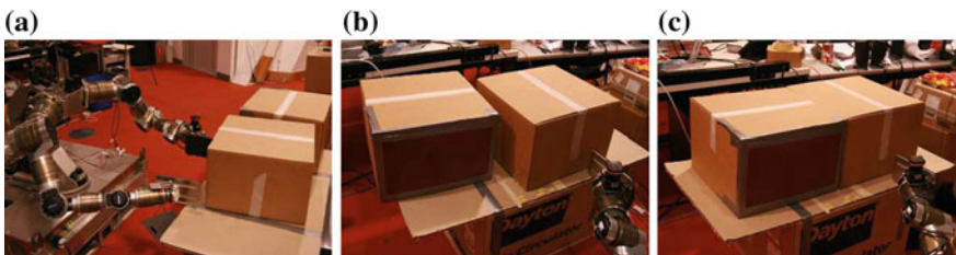
Fig. 3 Illustration of the grasping problem (a). The robot must localize the pose and dimensions of the boxes using the laser scanner mounted on the left wrist. This is relatively easy when the boxes are separated as in (b) but hard when the boxes are pressed together as in (c)
