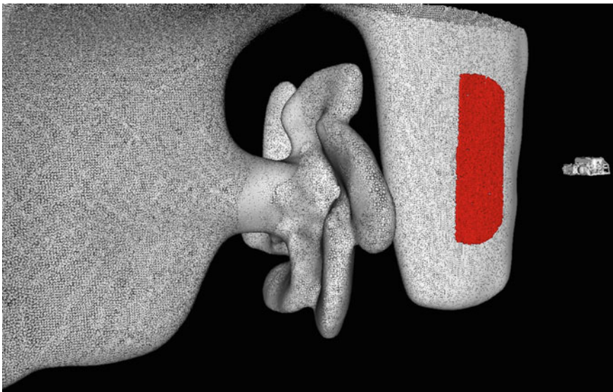
Fig. 4 A polygonal mesh obtained from our original, safe-distance survey of the SS Curtiss is depicted. The HAUV is illustrated in a configuration from which it observes a portion of the ship’s rudder. The red patch shows mesh points imaged at a desired sensor range between 1 and 4 m, as the sonar sweeps through 180° pitch. The ship mesh contains 107, 712 points and 214, 419 triangular faces. The propeller is approximately 7 m in diameter
