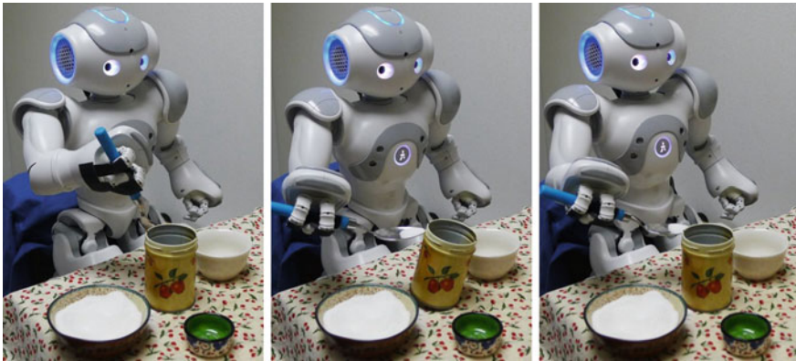
Fig. 1 We consider the household task of using a spoon to transfer sugar from a bowl to a cup on a table. Using standard motion planning algorithms without explicitly programming task constraints will fail since the spoon will not be kept level, causing the sugar to be spilled on the table ( left ). Methods based on learning from demonstrations are often unable to compute collision-free trajectories when novel obstacles are introduced in new locations not considered in the demonstrations ( middle ). Our method effectively combines motion planning with learning from demonstrations to avoid obstacles and keep the spoon level to successfully transfer the sugar ( right )
