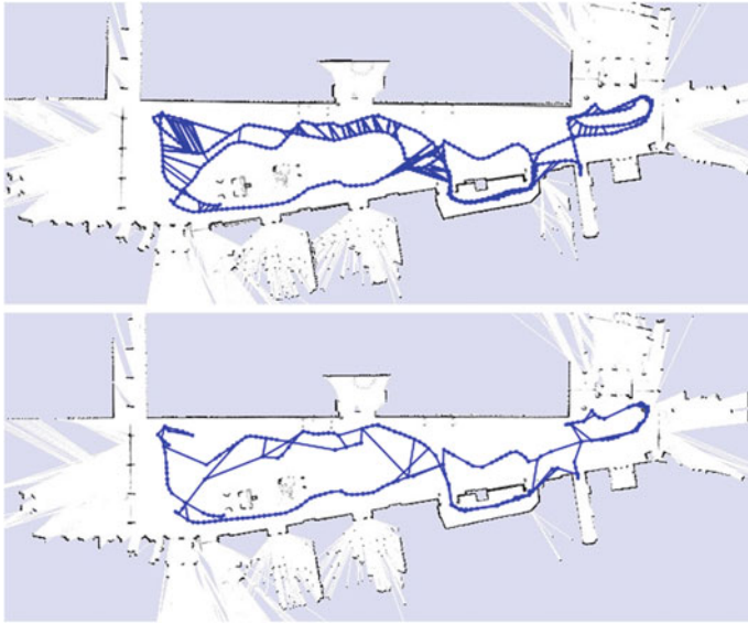
Fig. 4 Obtained map and pose graph for the FR101 dataset ( top standard approach, bottom our approach). Since the robot does not frequently re-traverse known terrain, few scans were discarded (200 vs. 408 nodes and 246 vs. 723 edges)
