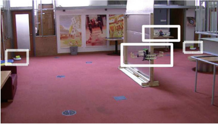
Fig. 1 Multi-agent field test environment with Ascending Technology Pelican quadrotors ( solid outlines ) and stationary ground sensors ( dashed outlines ). Infeasible regions include the wall in the center of the room, an open staircase that is partially visible on the right , and a table (out of view)
