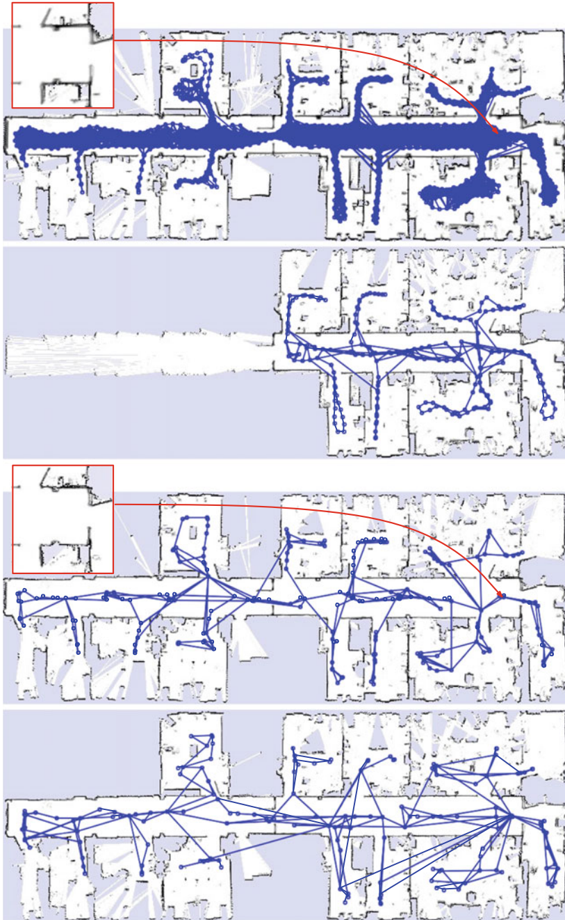
Fig. 3 The robot moved around in an office environment for an extended period of time, visiting the rooms and the corridor many times. First Standard approach, 2597 laser scans, 15695 edges Second Our approach at an intermediate time step, 200 laser scans, 264 edges. Third Our approach, 200 laser scans, 315 edges. Fourth Our approach when setting a threshold for the mutual information, 148 laser scans, 250 edges
