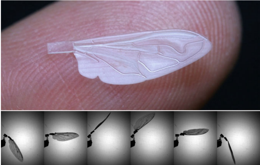
Fig. 6 Photo of a micromolded polymer wing mimicking the features of a Eristalis wing ( top ). This wing was created in a single molding step and includes veins ranging from 50 to 125 \mu\text{m} thick, 100 \mu\text{m} corrugation, and a 10–20 \mu\text{m} membrane. A sample of the wing motion (dorsal perspective) at 150 Hz flapping frequency taken from a high speed video ( bottom )
