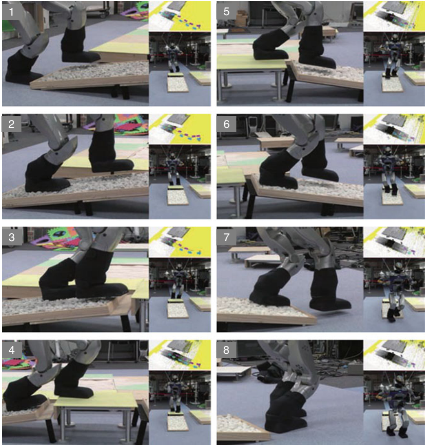
Fig. 12 Photographs of an experiment on autonomous navigation over unknown terrain (GUI)
