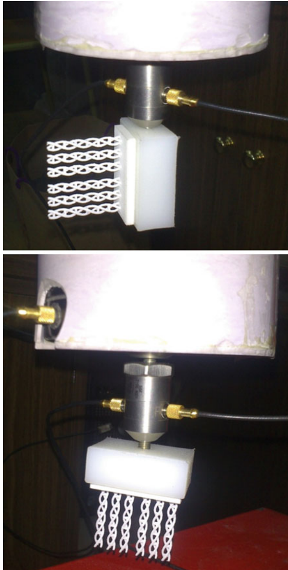
Fig. 14.8 Testing of the dynamic properties of polyamide prototypes of helical scaffolds for tendon and ligament repair obtained by selective laser sintering. Transversal excitation for the promotion of bending modes ( upper image ). Parallel excitation of the promotion of the axial modes ( lower image )
