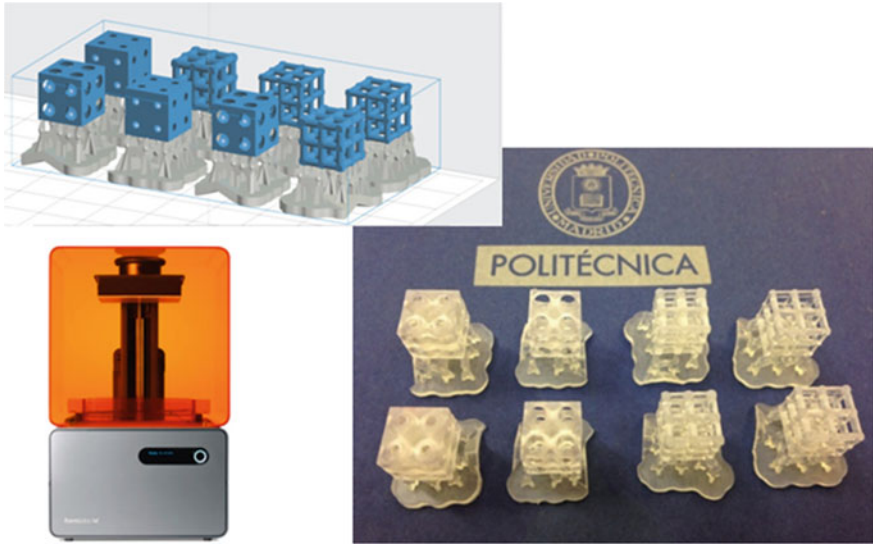
Fig. 8.9 3D designs and prototypes of different porous and lattice structures with potential application as tissue engineering scaffolds. Prototyping has been accomplished with a Form1+ machine from Formlabs
