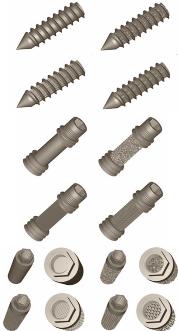
Fig. 17.4 CAD library of trabecular dental implants based on the concept of the tissue engineering scaffold applied to conventional prostheses (Within Lab software, trial version: http://www.withinlab.com/ )
