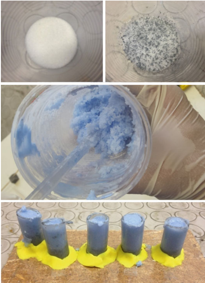
Fig. 19.2 Sugar and sugar mixed with SiC powder for their use as porogens towards the manufacture of functionally graded porous PDMS (blue) scaffolds (color online)
