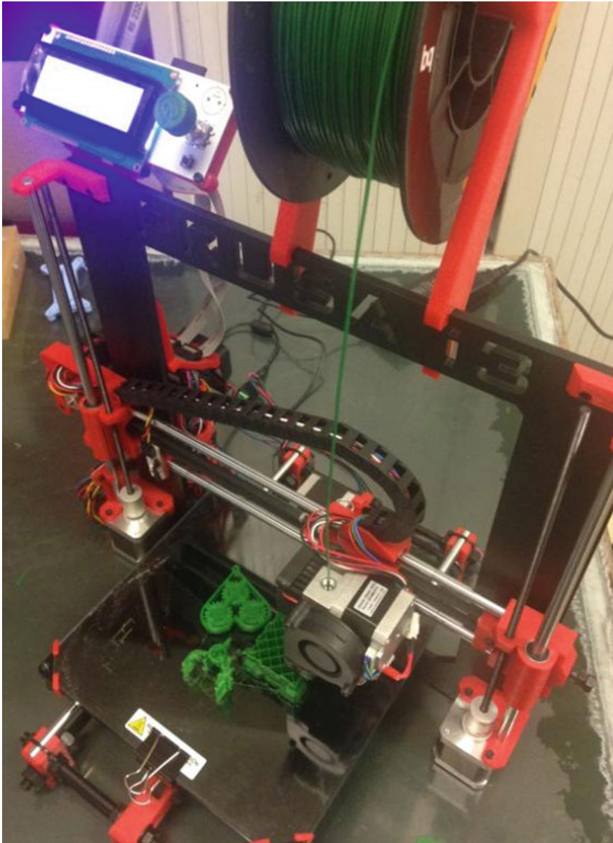
Fig. 15.8 Low-cost fused deposition modeling “Prusa Hephestos i3” machine for the production of rapid prototypes using thermoplastics such as PLA
