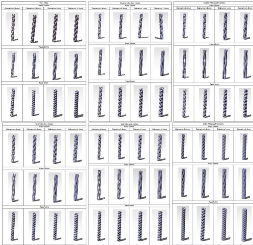
Fig. 18.10 Systematic computer-aided design library of DNA-inspired helical tissue engineering scaffolds for tendon and ligament repair
