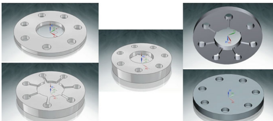
Fig. 11.4 Different 3D CAD models of a biomedical microsystem for disease diagnosis actuated by capillary action
