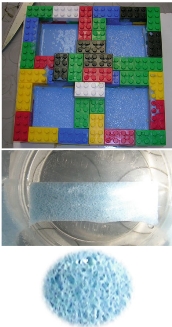
Fig. 18.3 Development of biomimetic porous PDMS for mimicking cartilage by means of casting PDMS-sugar mixtures into rapid molds and final particle leaching by water immersion after polymerization
