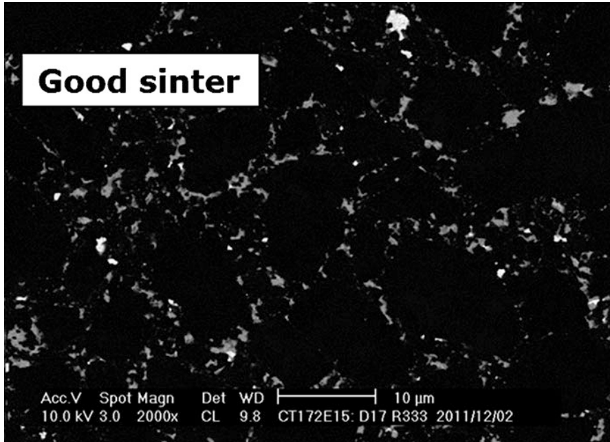
Fig. 2.12 Showing well-sintered PCD material (courtesy of E6)
