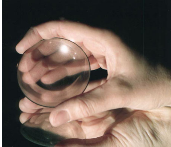
Fig. 2.24 A polished CVD diamond dome
