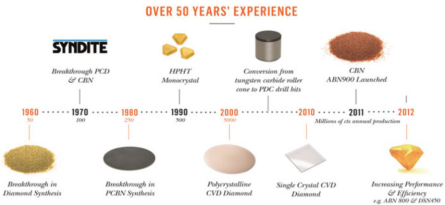
Fig. 2.2 The development of synthetic diamond and CBN materials (courtesy of Element Six (E6))
