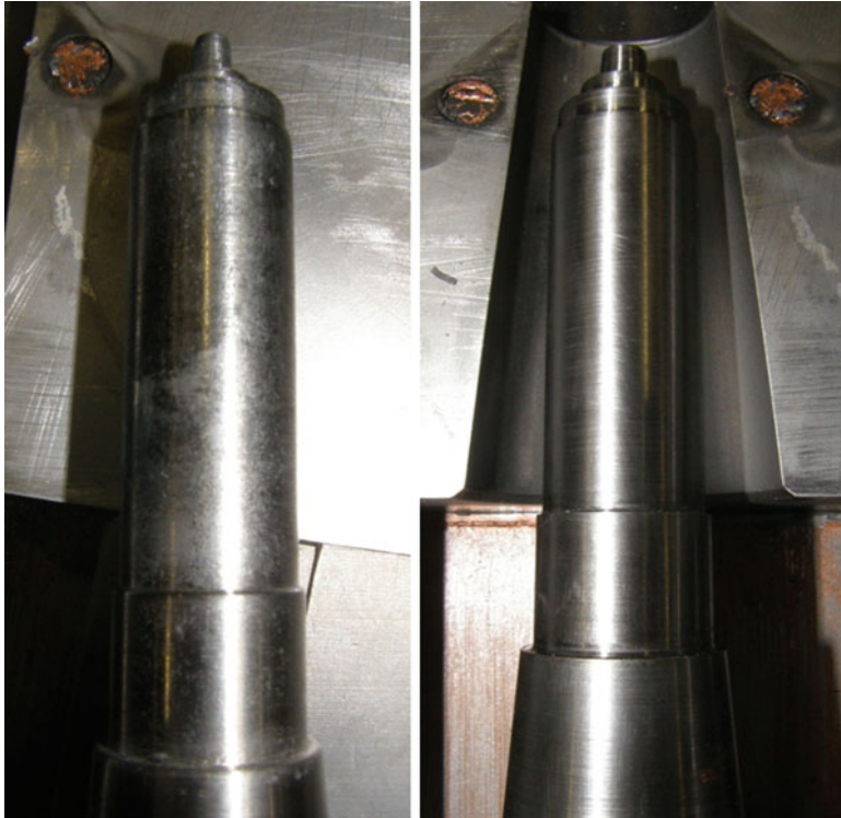
Fig. 6.20 Tools for injection molding of Al alloys in fabrication of parts for automotive industry, both after the fabrication of 15,000 parts. The length and diameter of the tools are about 200 and 20 mm, respectively. Left tool with conventional surface treatment by nitriding, right tool coated with 2–3 \mu\text{m} thick nc-( \text{Cr}_{1-x}\text{Al}_x )N/Si 3 N 4 coating [From SHM, private communication (2013)]
