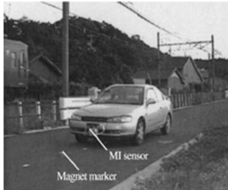
Fig. 8.12 Automated highway system (AHS) experiment with a MI sensor: this car drives automatically without a driver (reprinted with the permission of Elsevier [2])
