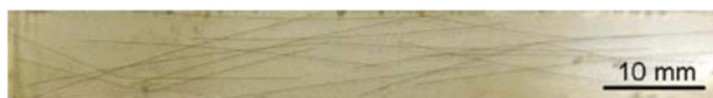
Fig. 11.24 Image of the composite sample containing 0.026 vol% microwires. Reprinted with permission from [75], copyright 2012 AIP
