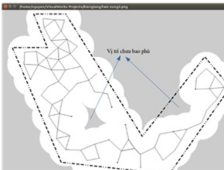
Fig. 9. The representation of the areas that are not covered by the sensor network (1)
