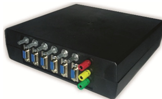
Fig. 4. Multichannel photoplethysmography device with three connectors for ECG electrodes. ECG in this device is used for time synchronization of all of pulse wave during one cardiac cycle.
