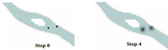
Fig. 8. The parallel simulation of diffusing pollution in a river. This is initialized with two polluted points (dark points).
