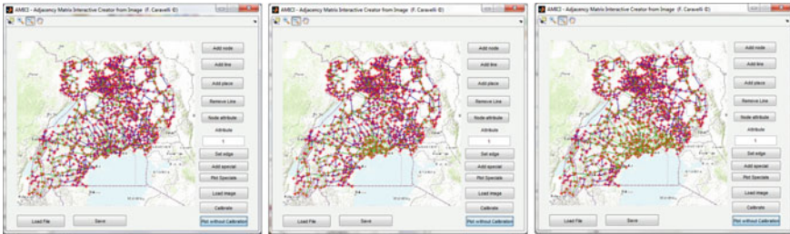
Fig. 20.6 Left current condition of road infrastructure in Uganda. Blue roads represent gravel roads meanwhile green are paved roads. Center A plausible infrastructure improvement policy for the road infrastructures around the cities of Kampala and Entebbe; each shipment has to pass through this area in order to reach exporters and the airport. Right A more substantial policy, where the improvement is extended also to the farming area where the agents of the model are located
