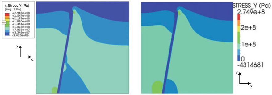
Fig. 9.12 Y component of the stress field (Pa) calculated ABAQUS (left) and OGS (right)
