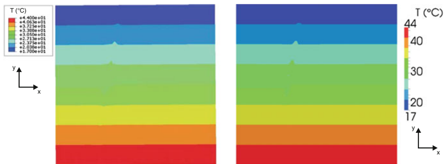
Fig. 9.14 Temperature (°C) calculated with ABAQUS ( left ) and OGS ( right ). Temperature increase (decrease) can be observed in the fold as a result of fluid outflow from the storage aquifer into the fault
