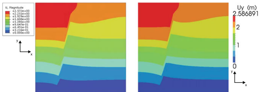
Fig. 9.11 Displacement in the y direction (m) calculated with ABAQUS ( left ) and OGS ( right )
