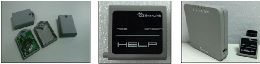
Fig. 2. a. (left) Customizable object and human sensors prototype; b. (center) The SOS alarm prototype; c. (right) The Home Gateway prototype.
